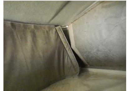
**E** - Start with the front part, followed by the rear part and the two side parts. The stitched Velcro tape allows the attachment of the insulation directly to the headlining material. Ensure that the locking mechanisms are positioned in front of the insulation mat.
