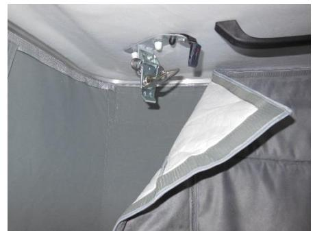
**E** - Please take note of the size and form of the 4 individual parts. The rear section is narrow and short. The two side sections are of equal length and constitute the two longest parts of the sleeping roof insulation, having a shape similar to a triangle. For an additional attachment, fix the additional self-adhesive fleece stickers all round to the lower frame.
